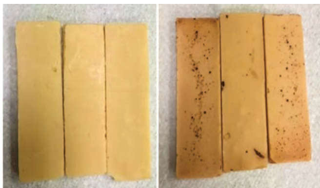
FIG. 3. Epoxy before immersion (left) and after 30 d of immersion (right).
