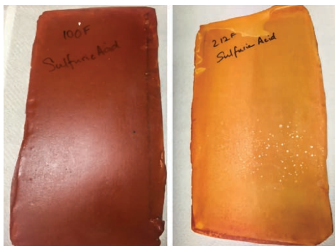
FIG. 5. Composite panels after 1,000-hr of immersion and then cured at 38°C (100°F) for 17 hr (left) and cured at 100°C (212°F) for 6 hr (right).
