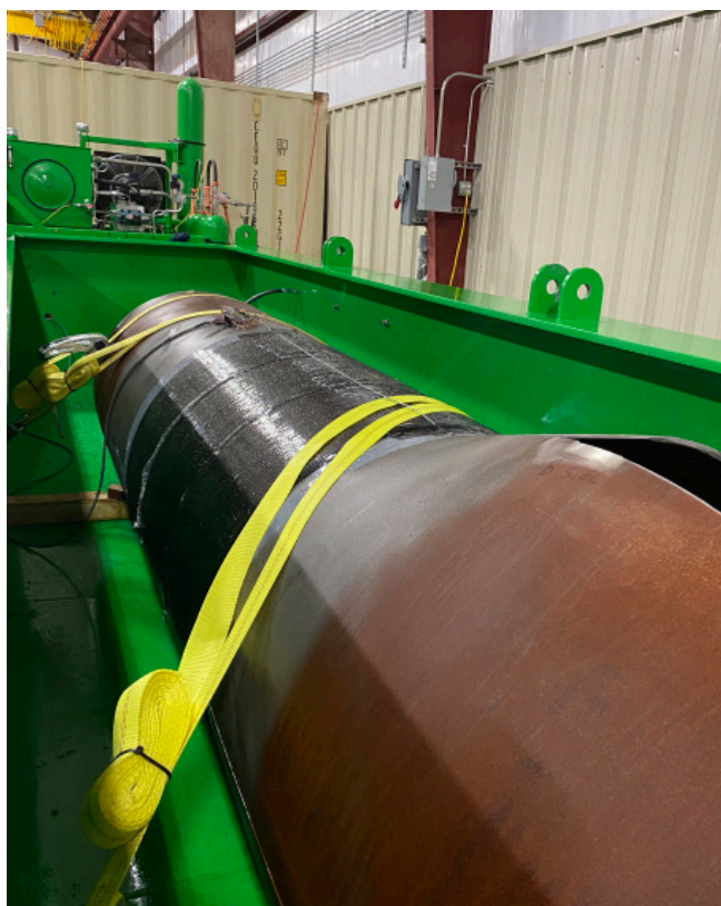
Figure 2. Atlas was validated on seam weld defects manufactured on full-scale spool tests.
