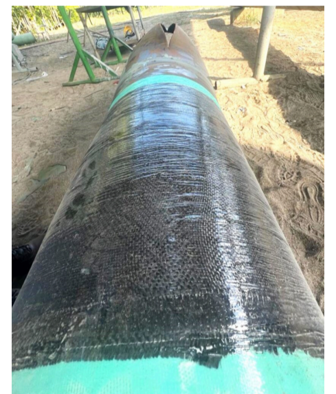
The burst test revealed that the Atlas system outperformed all other non-metallic reinforcements for repairing pipe with wall loss of up to 80%.
